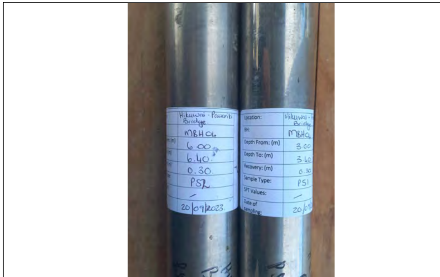
Photo MBH 04.13 Push tube sample depths
