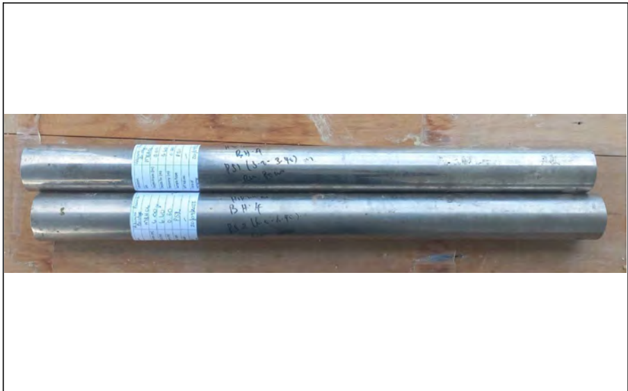
Photo MBH 04.12 Push tube samples
